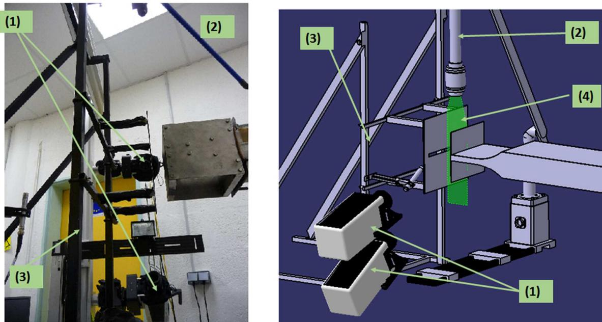
Figure 3: Stereoscopic PIV Set-up
