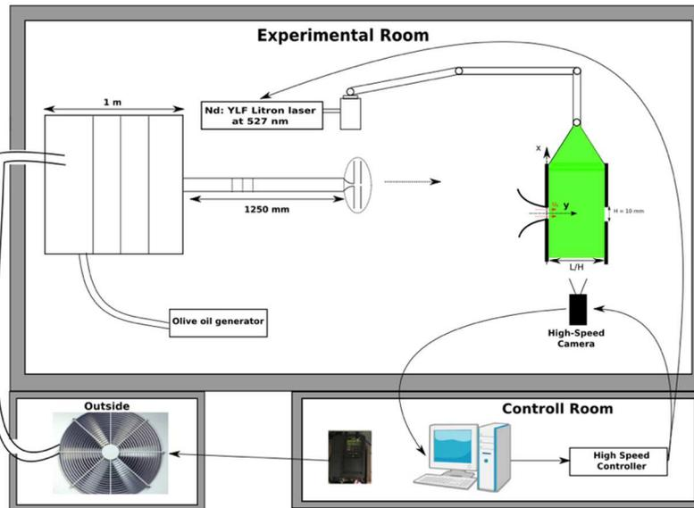
Figure 2: 2D-2C PIV Set-up
