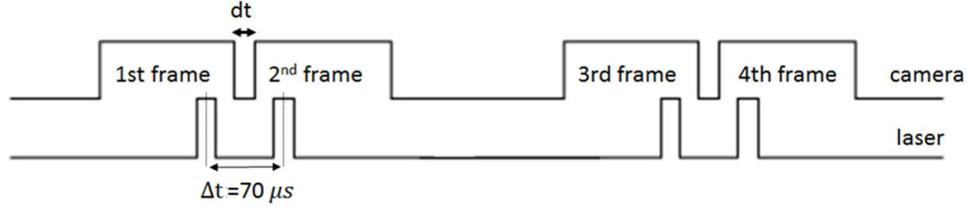
Figure 4: Signal diagram to synchronize camera and laser shutter
