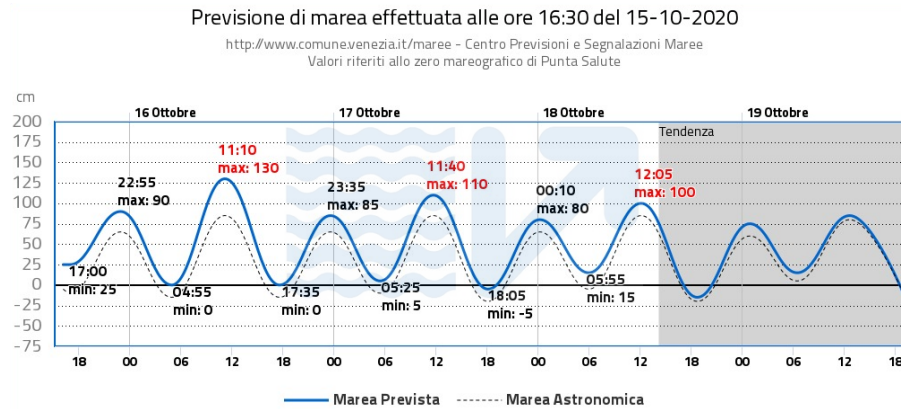
Figure 5. An example of the daily bulletin published on the official forecasts website of CPSM – Venice Municipality. The chart shows a 4 d forecast plus 1 d forecast trend. The water level refers to the Punta Salute datum, the historical zero of Venice defined in the year 1897. The blue line is the total expected sea level, and the dotted black line indicates the astronomical tide.
